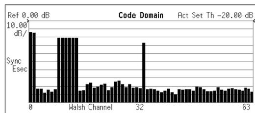
Figure 12. Two-carrier CDMA signal with code domain noise from baseband image
