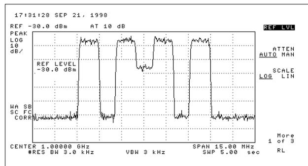
Figure 10b. Spectral plot of multicarrier CDMA signal
