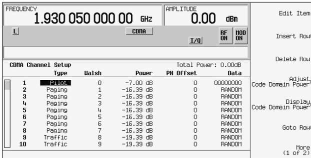
Figure 3. CDMA channel-table editor preloaded with 64-channel configuration
