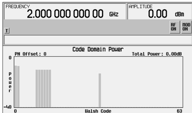
Figure 4. Code-domain power display for a 9-channel configuration
