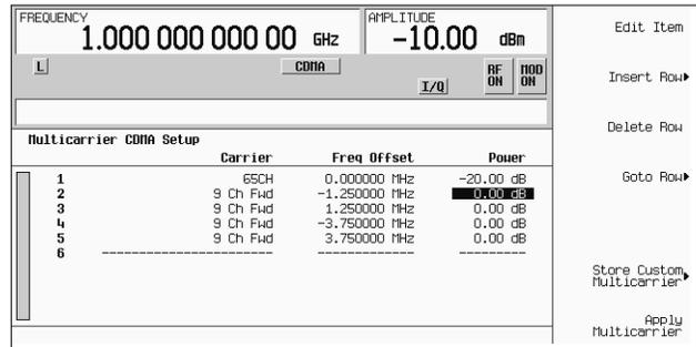
Figure 10a. Multicarrier CDMA custom configuration
