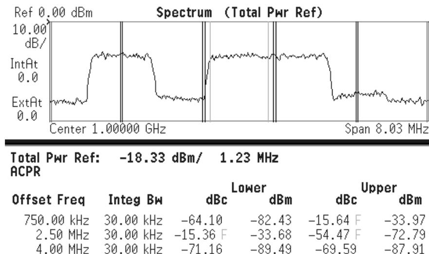
**Figure 11. Multicarrier CDMA signal with baseband images**
